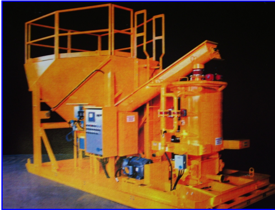
Cemented Rock Fill Slurry Mixer Plant
