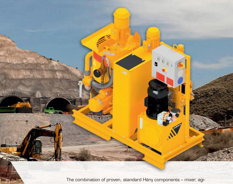
The combination of proven, standard Häny components – mixer, agitator, and injection pump – results in an extremely compact injection plant. This setup is suitable for a wide variety of applications such as anchor, sleeve pipe, and contact injections.
