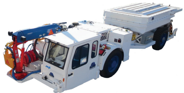
Aliva 302 Spray Boom and Aliva 257 Wet/Dry shotcrete machine assembled on a Carrier
