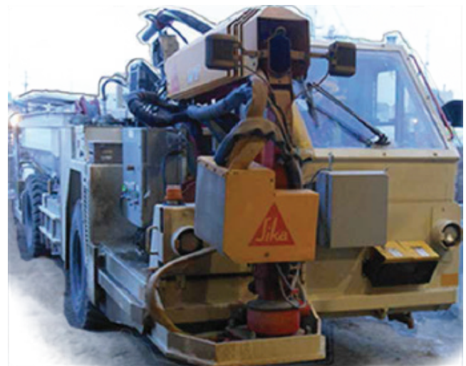
Aliva 302 Spray Boom and Aliva 257 Wet/Dry shotcrete machine assembled on a Carrier
