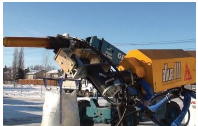
Aliva® 302 Spray Boom with 240/360 degree Nozzle Rotation
