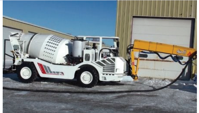
Aliva® 302 Spray Boom partially extended
