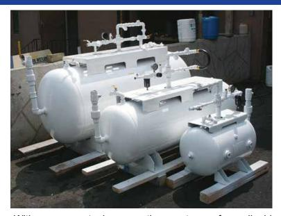
With pressure tank generating systems, foam liquid concentrate and water are premixed in the tank. The solution is then discharged from the pressurized tank through the foam-making nozzle. No additional water pump is required. The process is completed by air pressure alone.
