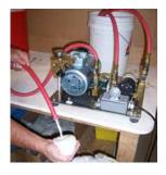
There is also a portable lab foam generator for producing accurate mix design results in the laboratory.
