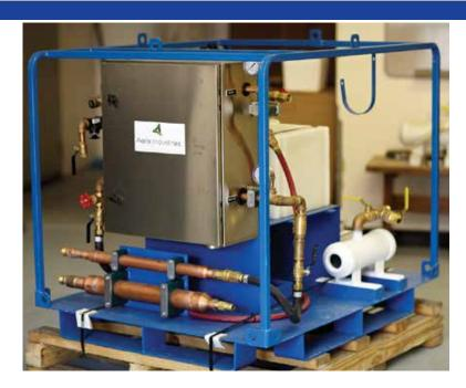
Our Auto-Foam Generator (AFG) automatically blends liquid foam concentrate with water and compressed air in fixed proportions. The AFG continuously siphons liquid foam concentrate directly from the concentrate's container. The liquid foam concentrate is metered and blended with water yielding a premixed solution with the proper concentration ratio to produce the desired density.
