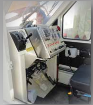
Operator Drive Compartment ROPS / FOPS Certified
