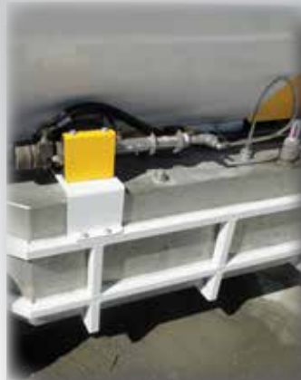
Liquid Accelerator Tank and Dosing System
