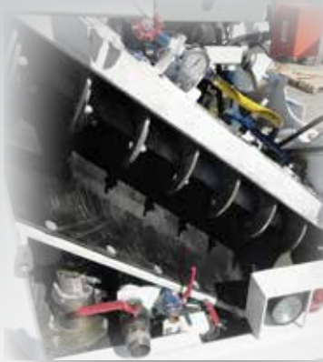
Hybrid-Wet Shotcrete® Easy-Clean Mixing Chamber
