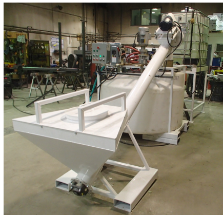
Liquid Shotcrete Accelerator Mixing station and storage
