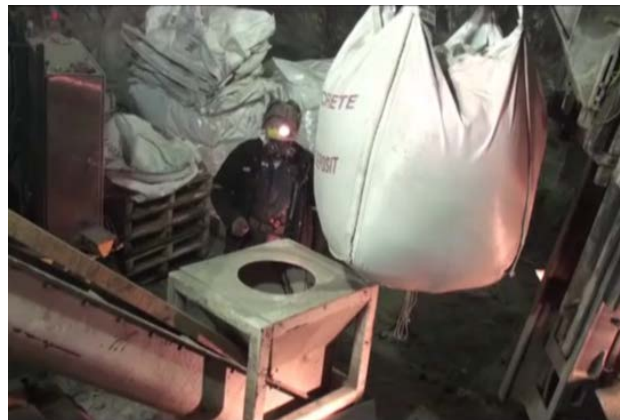
Unload feed hopper - for bulk dry material
