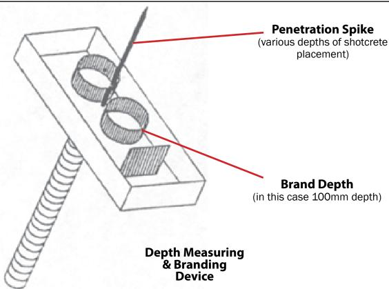
Multicrete Shotcrete Depth Measuring Device Branding System has an easy-reach system.
