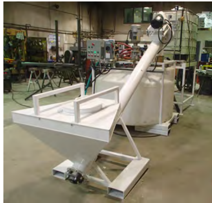
Liquid Shotcrete Accelerator Mixing station and storage
