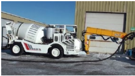
Aliva 302 Spray Boom Partially Extended
