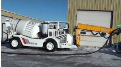
Aliva 302 Spray Boom Partially Extended
