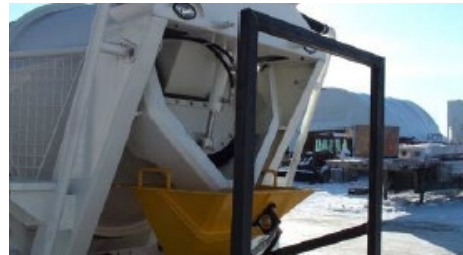
Drum discharge chute to Aliva 257 Hopper
